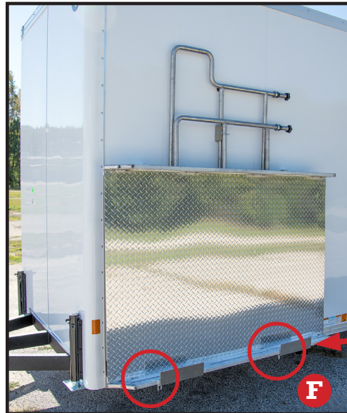
Center ADA ramp on Base with top side facing outward. See image F .
